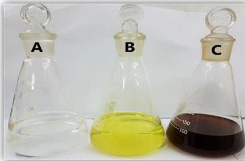
**Fig. 3:** (A) The colorless solution of  $\text{AgNO}_3$ , (B) The solution of AgNPs prepared from methanolic extract of *Gracilaria parvispora* after 15 minutes, (C) The solution of AgNPs after 90 minutes.
