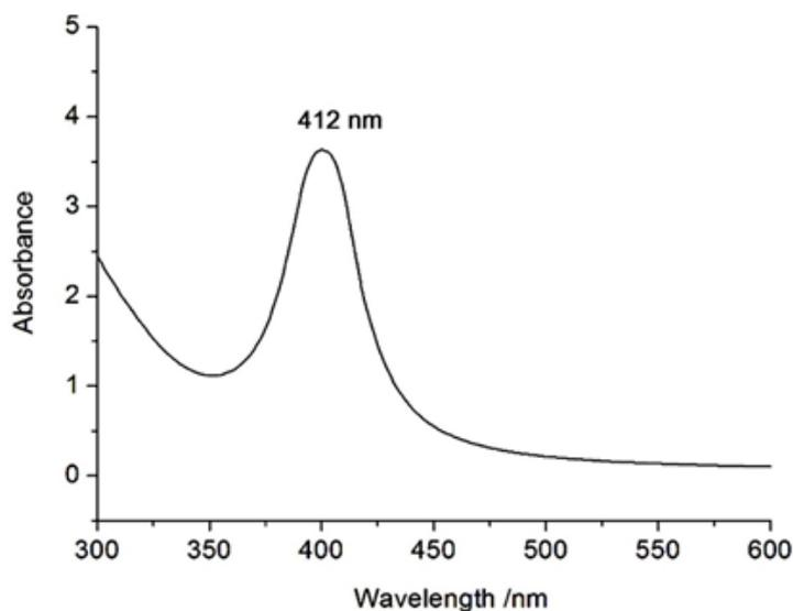
**Fig. 4:** UV–Visible spectrum of silver NPs synthesized by *Gracilaria parvispora* extract.
