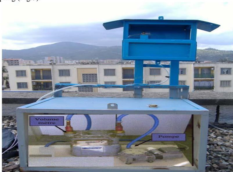
Fig. 2: Low volume sampler LVS
