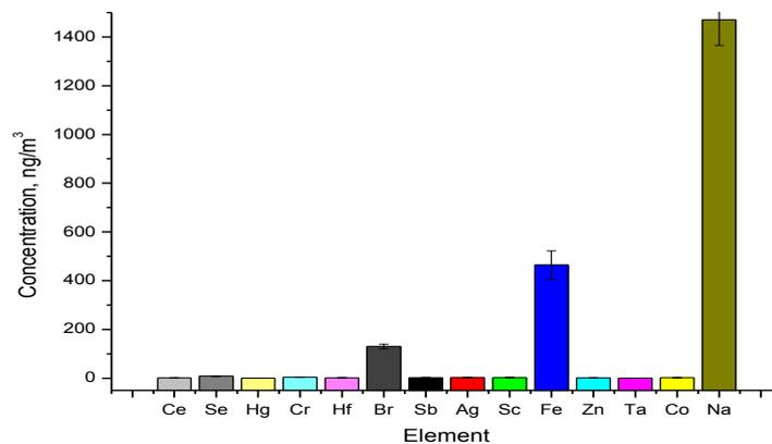
**Fig. 9:** Concentration of elements analyzed by INAA in air filter sample of air (Irradiation time 6h) at the Haute Casbah.
