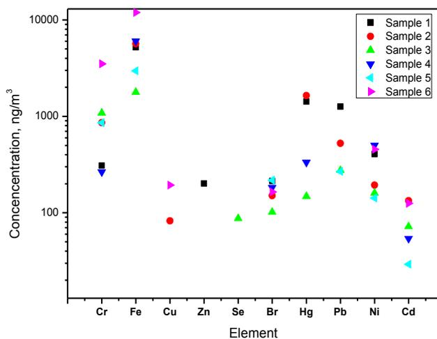
**Fig. 7:** Concentration of elements analyzed by EDXRF in air filter samples collected at CHU Bab El Oued.
