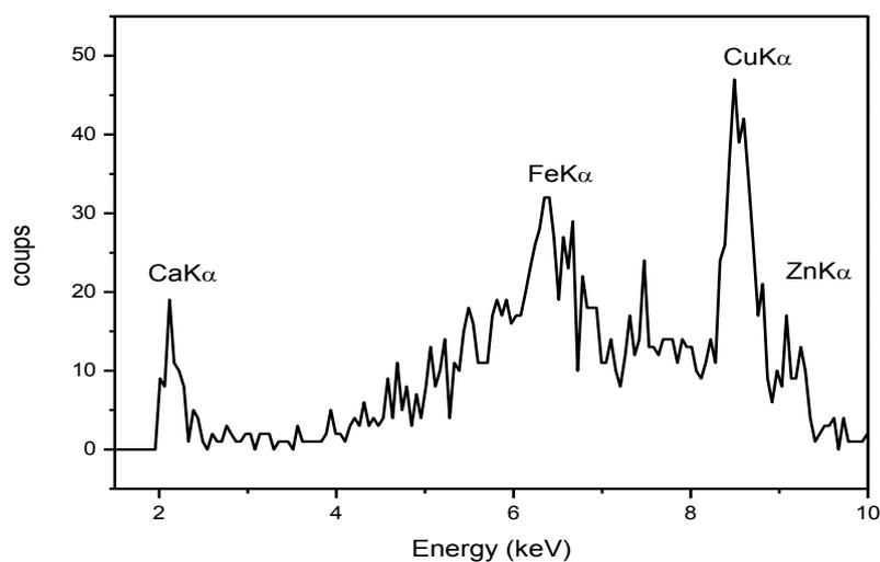
**Fig. 5:** Spectrum PIXE of air filter sample at 2 MeV protons beam energy.
