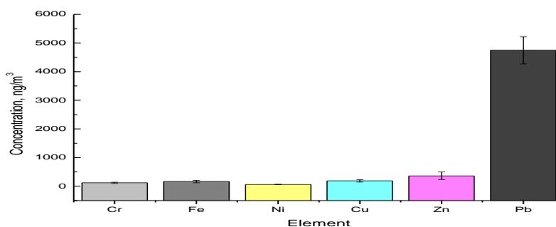
**Fig. 6:** Concentration of the elements analyzed by PIXE in air sample filters collected at the Haute Casbah.
