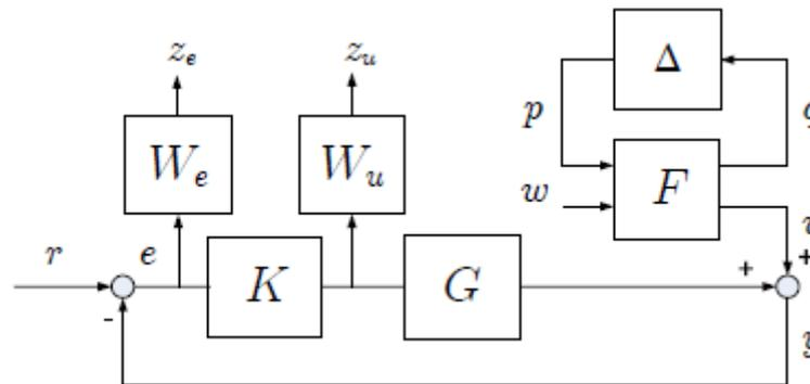
Fig. 4: System interconnection for the disturbance rejection problem Consider the interconnection in Figure 4 in which  $G$  is the plant model given as
