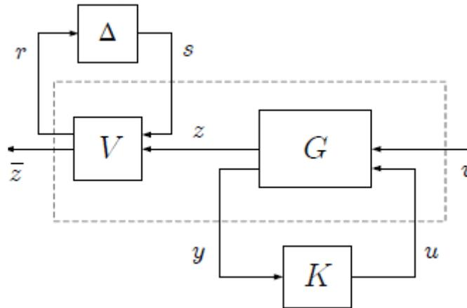
Fig. 3: System interconnection corresponding to generalized plant
