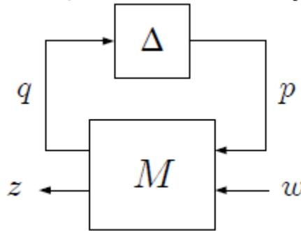
**Fig. 1:** Interconnection for Stability And Performance Analysis
