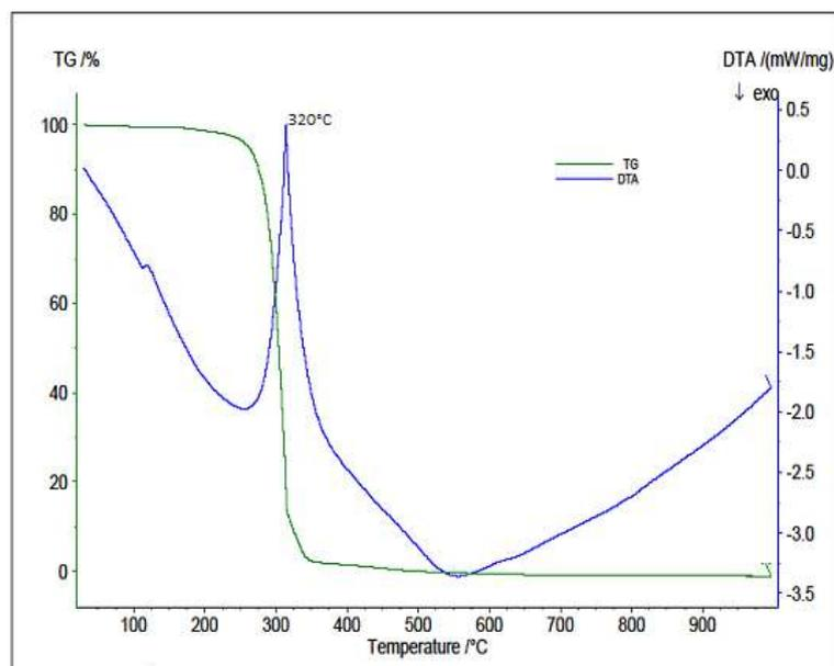
**Fig. 7:** TGA-DTA curve of MND crystal
