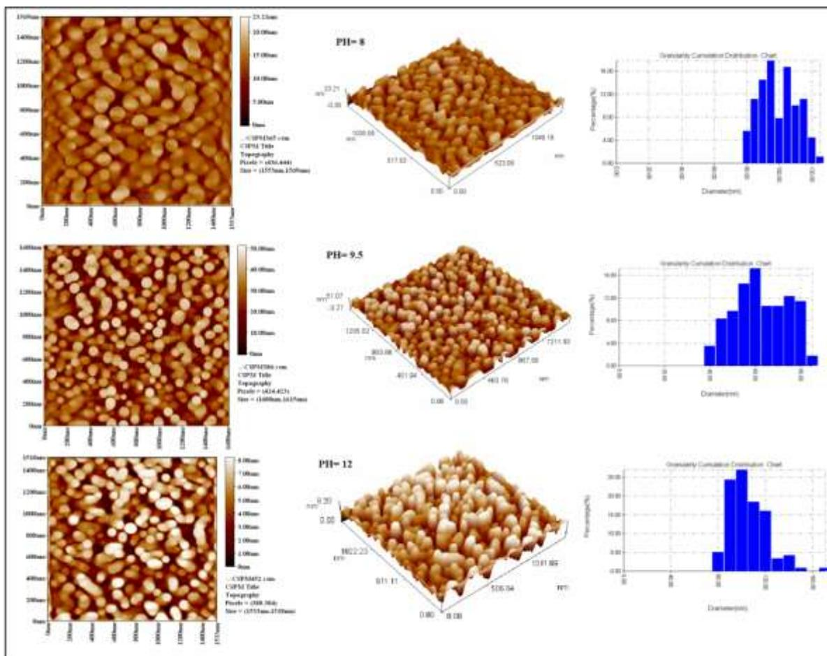
**Fig. 2:** AFM measurement of ZnS NPS surface deposited on glass substrate and for different pH and their granularity accumulation distribution of ZnS films.
