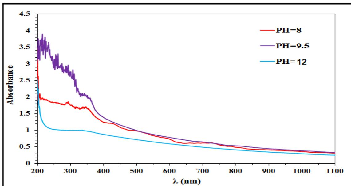
Fig. 4: UV-VIS absorption spectrum of ZnS nanoparticles films for different pH on glass substrate.
