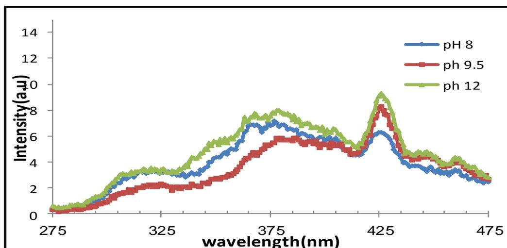
Fig. 5: PL spectra of the ZnS colloidal for different pH of solution.
