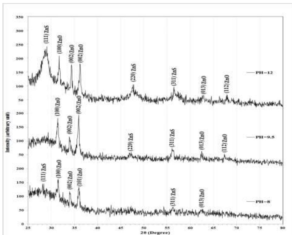
**Fig. 1:** The XRD pattern of the ZnS nanoparticle.
