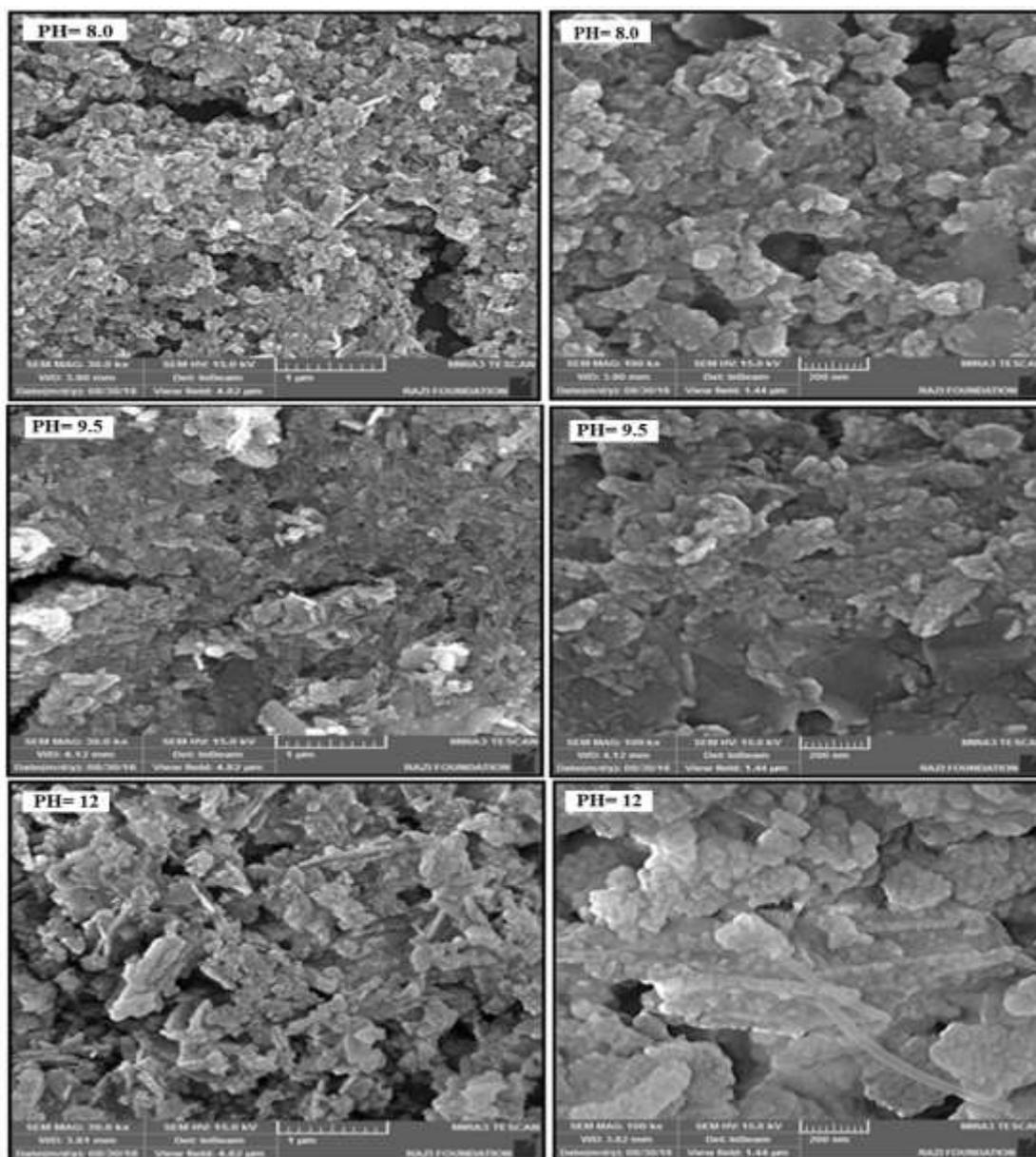
**Fig. 3:** ZnS nanoparticles samples by FESEM with (a) low magnification (left), (b) high magnification (right).
