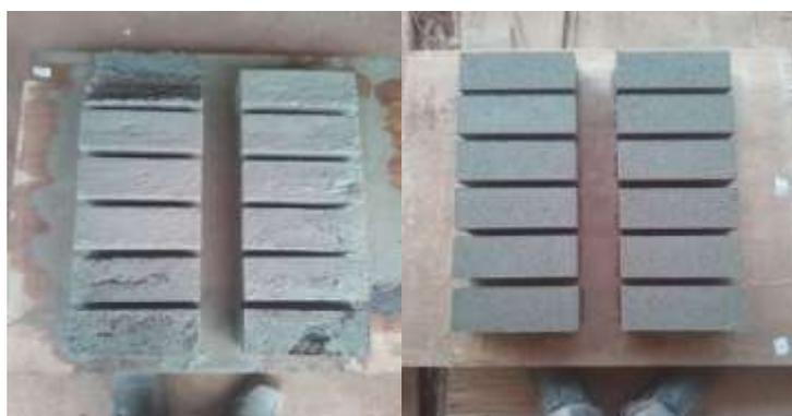
**Fig. 5:** 0.5w/c **Figure 6:** 0.45w/c
