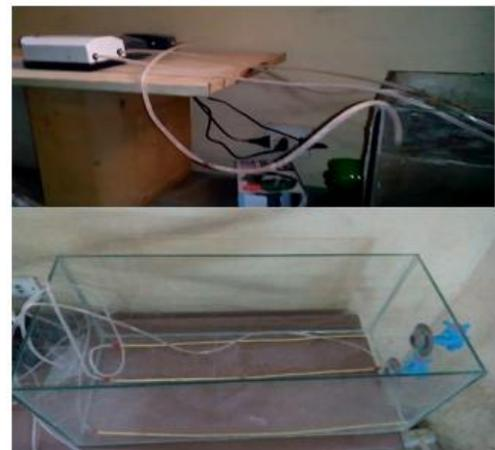
A pilot was made by a 30 \* 30 \* 60 cm aeration tank with a total volume of 54 liters with a working capacity of 45 liters, with a freeboard capacity of five cm. A diffuse air system that uses three air tubes mounted at the bottom of the reactor to pump air into the tank to add ventilation cycles. The design for the pilot and the real pilot components is shown in Figure no. (1).
