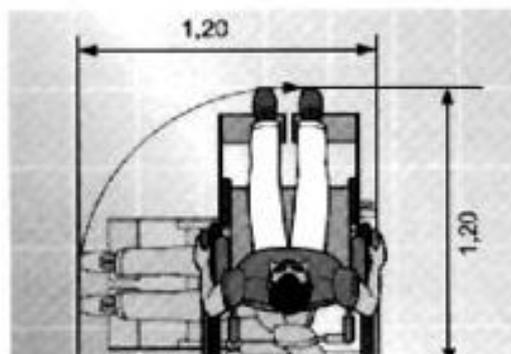
Figure 3: Rotation maneuver without frontal displacement.
