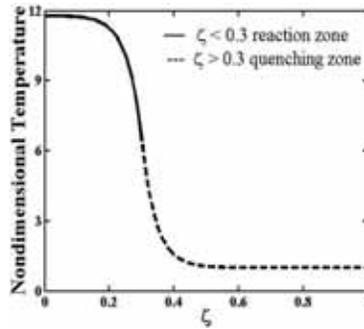
Fig. 2: Profile temperature as quenching plates width ( $d_p = 5.4 \mu m$ ,  $\tau_p = 10^{-3} s$  , ).
