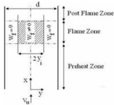
Fig. 1: Schematic diagram of the quenching plates.
