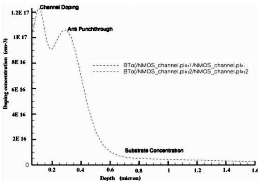
Fig. 1: Doping concentration profile versus depth in substrate.
