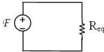
Fig. 4: The equivalent circuit of the permanent magnet model.
