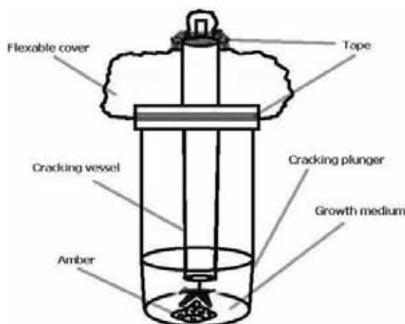
Fig. 2: The amber cracking vessel.
