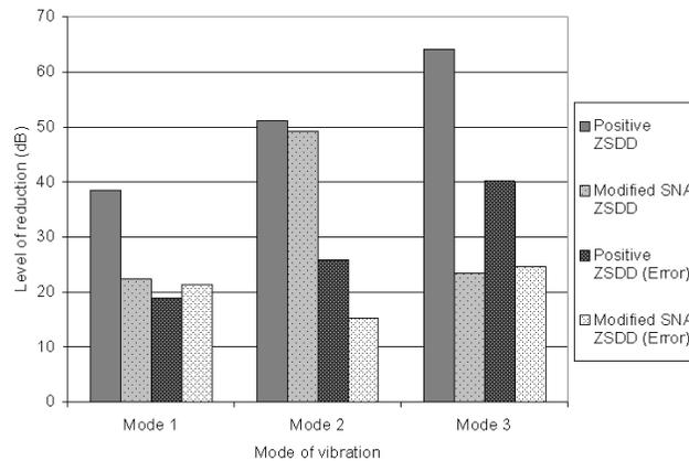
**Fig. 10:** Level of sway reduction with exact and erroneous natural frequencies with hybrid controllers.
