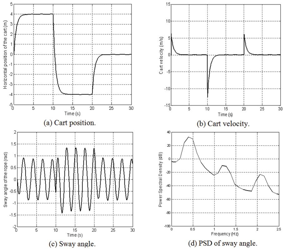
**Fig. 5:** Response of the gantry crane with LQR controller.
