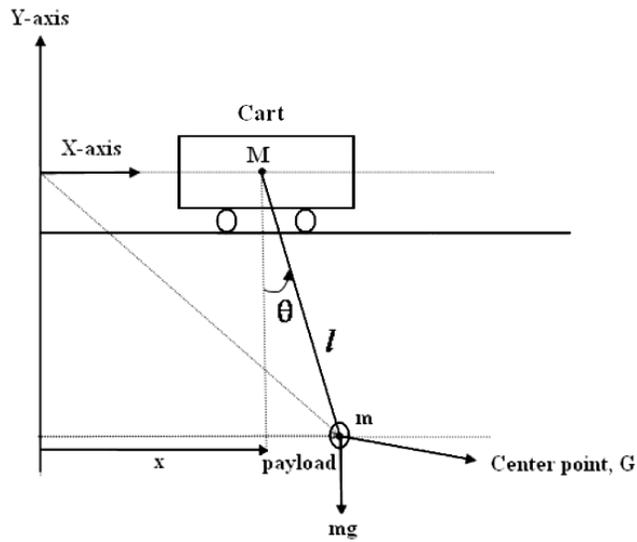
**Fig. 1:** Description of the gantry crane system.
