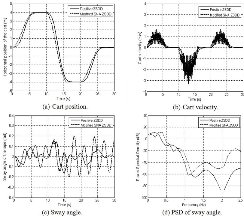
**Fig. 8:** Response of the gantry crane with hybrid controllers with exact natural frequencies.
