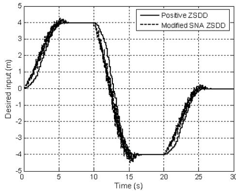
**Fig. 7:** Shaped inputs with exact natural frequencies using positive ZSDD and modified SNA-ZSDD shapers.
