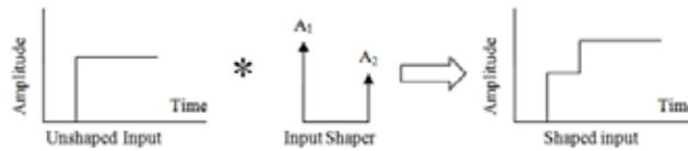
**Fig. 2:** Illustration of input shaping technique.
