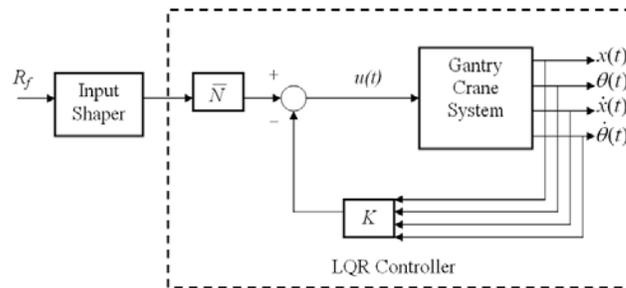
**Fig. 6:** Block diagram of the hybrid control schemes configuration.
