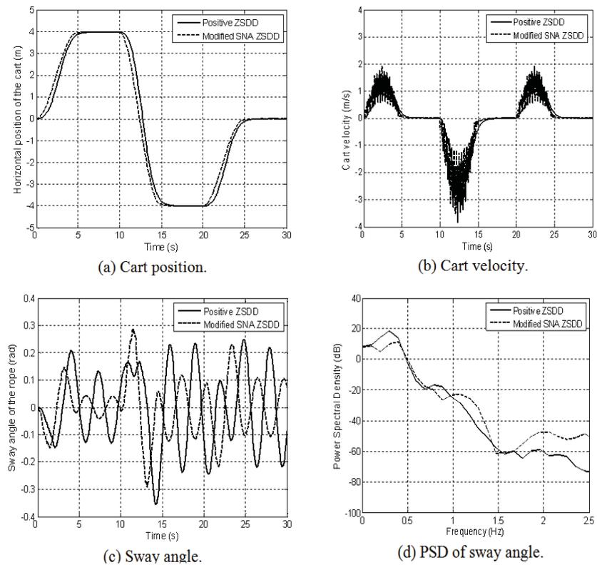
**Fig. 9:** Response of the gantry crane with hybrid controllers with erroneous natural frequencies.
