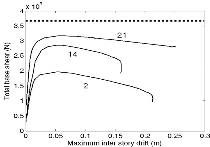
**Fig.7:** Total base shear as function of the maximum inter-story drift for combinations 2, 14 and 21
