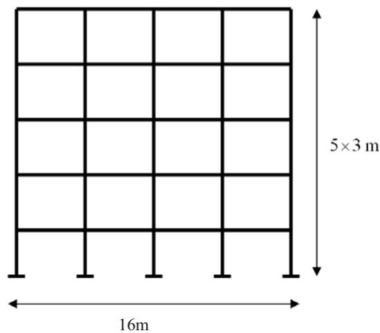
**Fig. 3:** Vertical elevation of the five-storey reinforced concrete structure in the seismic direction
