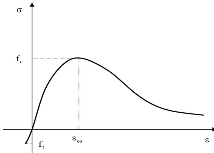
**Fig. 1:** Uniaxial constant confinement concrete model
