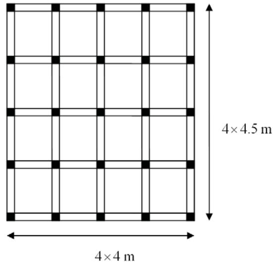
**Fig. 4:** Plane view of the five-storey reinforced concrete structure
