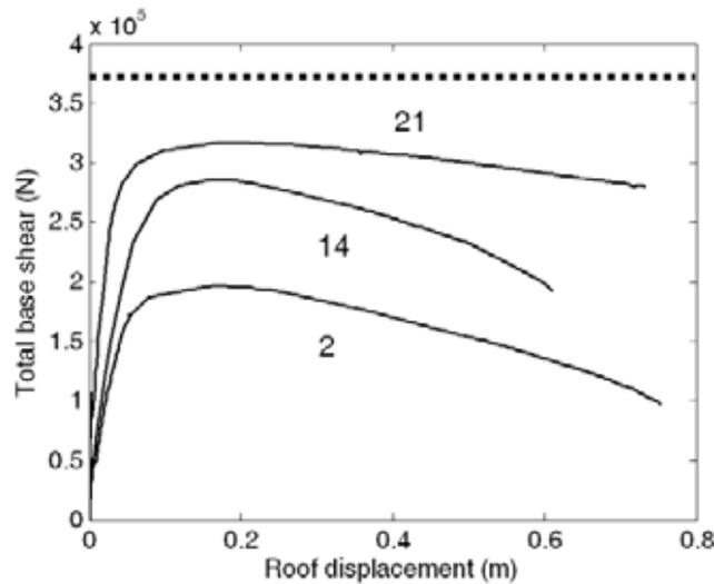
**Fig. 6:** Total base shear as function of the roof displacement for combinations 2, 14 and 21
