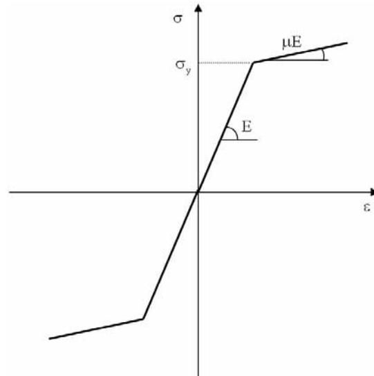
**Fig. 2:** Uniaxial bilinear elasto-plastic law with kinematic strain-hardening modelling mild steel
