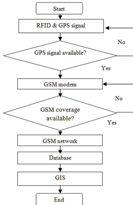
Fig. 2: System interface for bus monitoring
