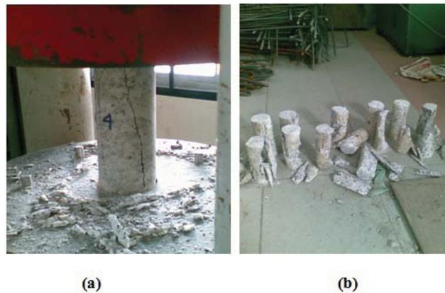
**Fig. 12:** (a) Sample is test until crushed to obtain peak strength (b) tested granite rock samples
