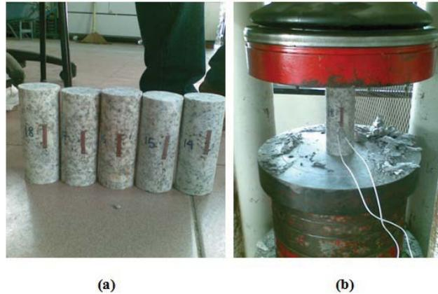
**Fig. 13:** (a) Radial strain gauges are attached to granite samples (b) 60% of average peak strength is applied using uniaxial compressive test (UCT)
