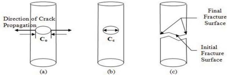
**Fig. 2:** Schematic diagram illustrating the process of fracture. (a) An initial crack of size  $C_0$ , (b) Crack propagation under the influence of a tensile load  $P$ ; the crack reaches a critical size  $C_c$  and the part becomes overloaded because of the corresponding reduction in cross-sectional area supporting the load. (c) Final separation due to an overloading condition. (Hani *et al.*, 2004).
