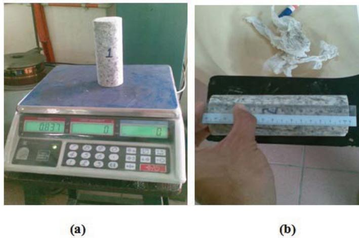
**Fig. 9:** (a) Weight of granite sample (b) Measurement of granite sample
