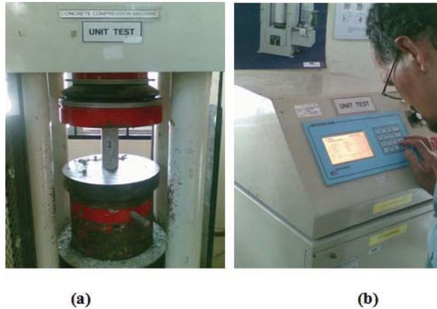
**Fig. 11:** (a) Uniaxial Compressive Test (UCT) (b) Uniaxial Compressive Test (UCT) result
