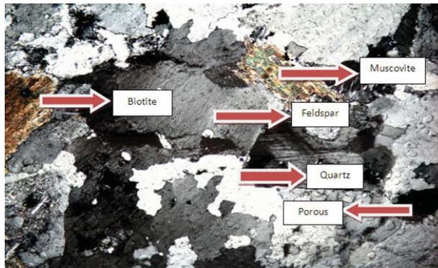
**Fig. 20:** The result for cross-polarised microscope (Sample-12).
