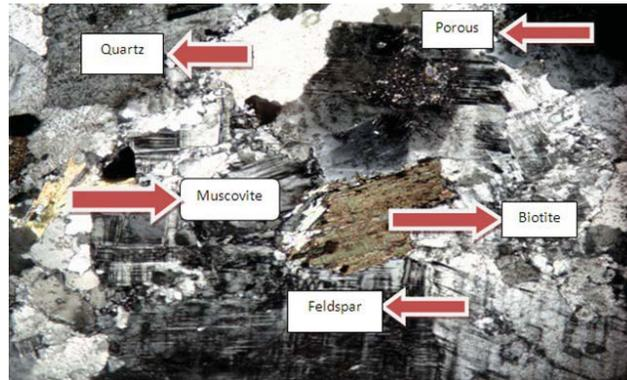
**Fig. 19:** The result for cross-polarised microscope (Sample-11)
