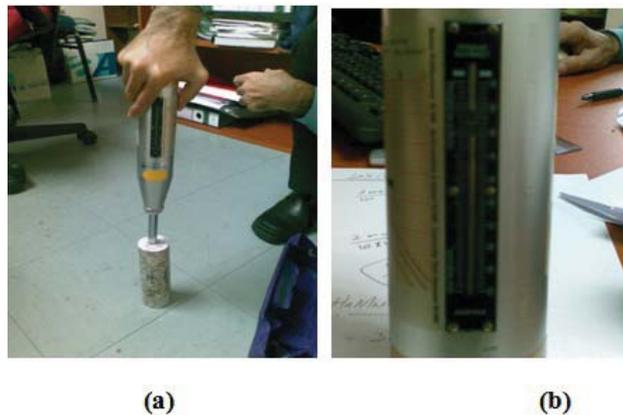
**Fig. 10:** (a) Schmidt Hammer (SH) (b) Schmidt Hammer (SH) reading
