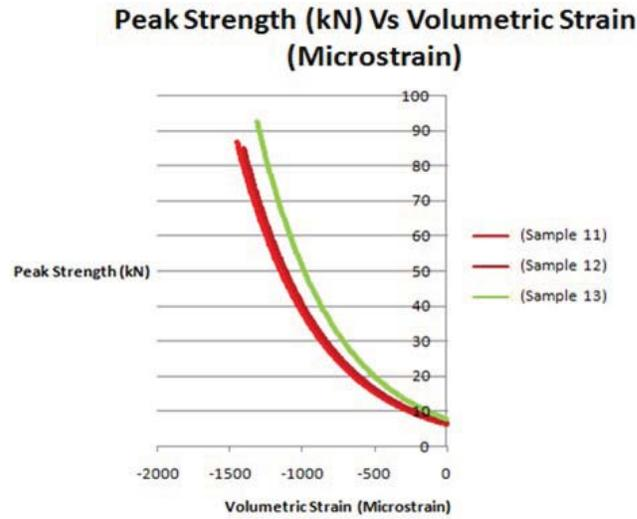
Fig. 17: Volumetric strain measured during uniaxial compressive test.
