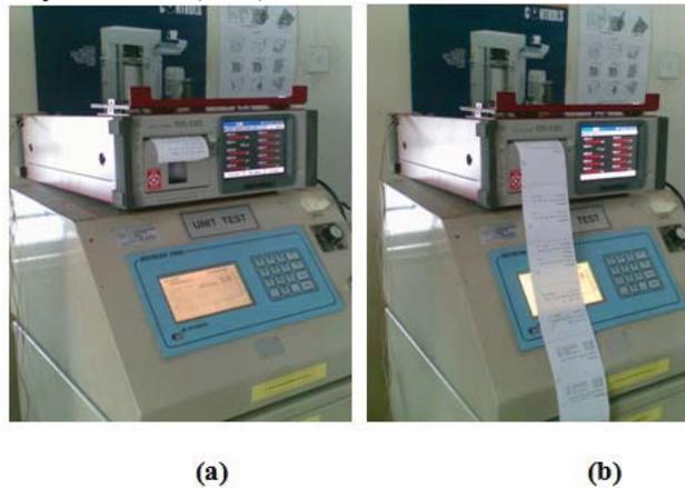
**Fig. 14:** (a) Radial strain gauge device (b) radial strain gauge reading
