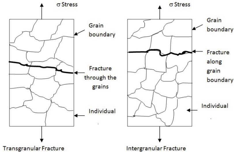
**Fig. 3:** Transgranular fracture (Pauzi, 2007)
