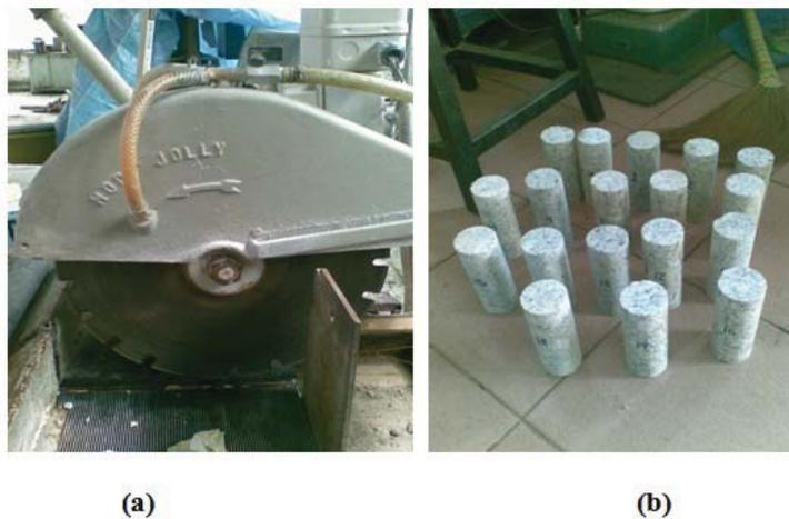
Fig. 8: (a) Diamond cutter machine (b) cutted granite rock 5 cm diameter and 15 cm height
