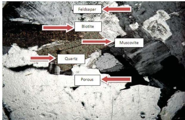
**Fig. 21:** The result for cross-polarised microscope (Sample-13)
