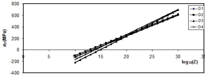
Fig. 1: Dependence of the maximum Stress on the Zener-Hollomon parameter.
