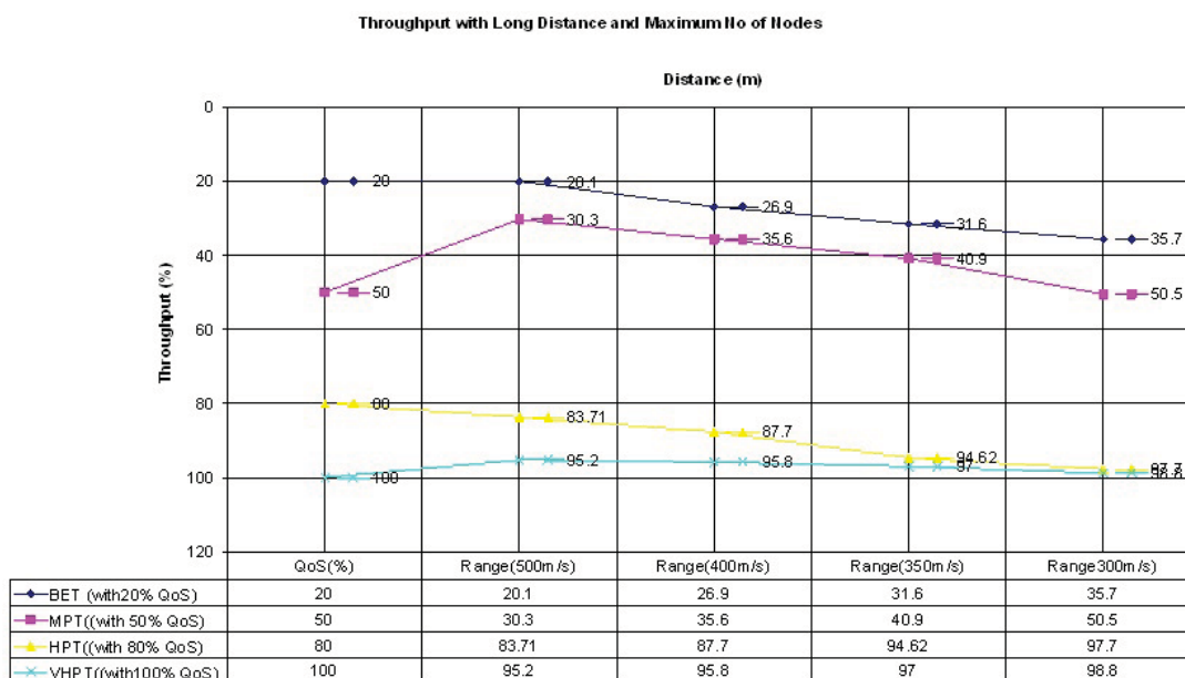
Fig. 4: Graph showing throughputs (End to End) when no of nodes are maximum (50) and distance is long from 300 – 500 meters
