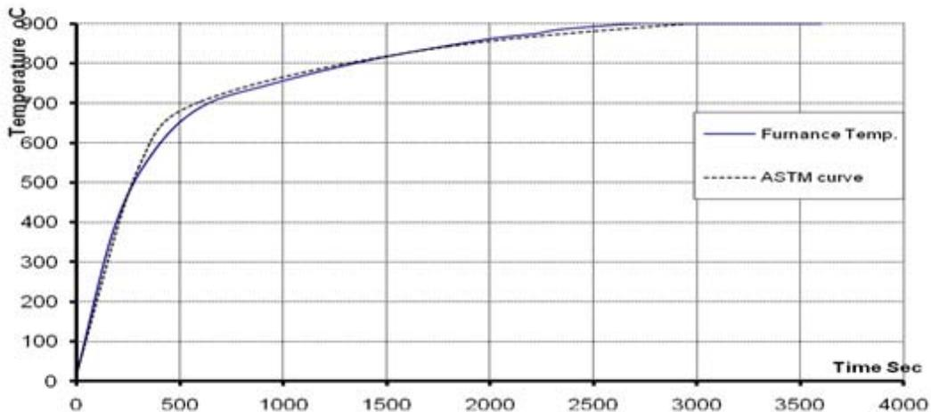
**Fig. 4:** Furnace Time-temperature curve, versus ASTM 119 fire test curve
