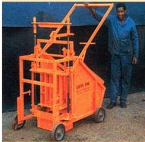
**Fig. 1:** Semi-Mechanized egg-laying machine
