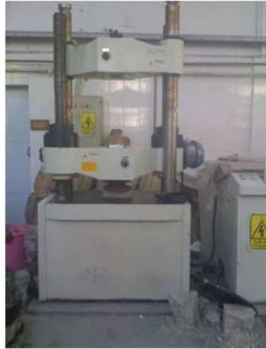
**Fig. 2:** The Shumadzu machine used for testing the rice straw-cement bricks
