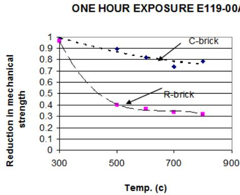
Fig. 5: One hour fire exposure test results for R and C-bricks
