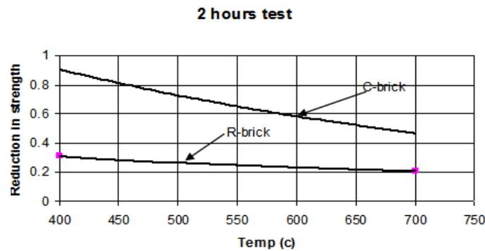
Fig. 6: Two hours fire exposure tests results for R and C-bricks
