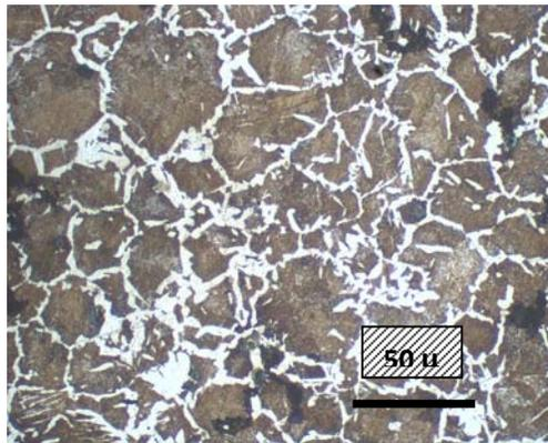
**Fig. 1:** The light microscope micrograph of quenched and tempered steel CK60, etched in 2% nital solution.
