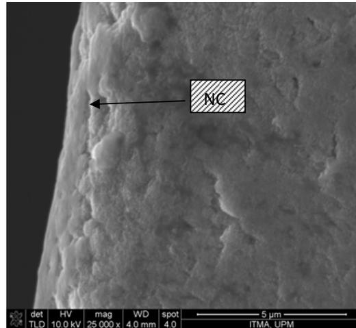
**Fig. 3:** The SEM Micrograph of CK60 steel drilled under 15 m/min speed.
