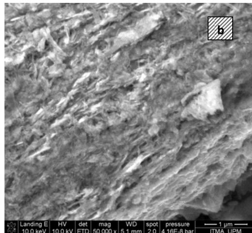
**Fig. 4:** The SEM Micrograph of CK60 steel drilled under 20 m/min speed. a)16000 X and b)50,000 X
