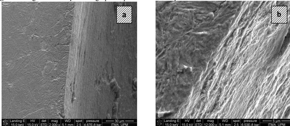
**Fig. 2:** A cross-sectional SEM observation of the CK60 steel drilled under 10 m/min. a) 2000X and b) 12000X
