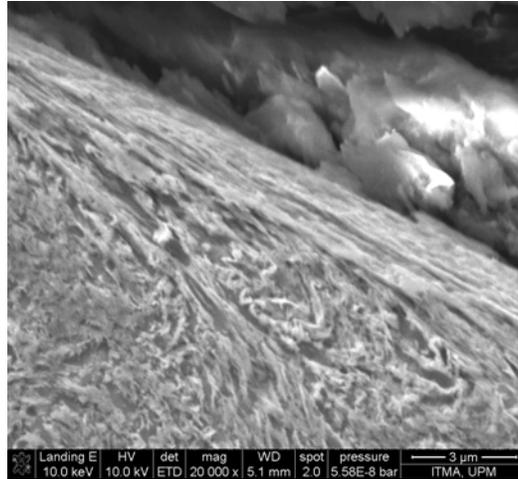
**Fig. 5:** The micrograph of sharp deformation angle – trace in sample drilled under 20 m/min speed.
