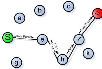
Fig. 6: Data flow in new route
