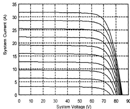
**Fig. 2:** Voltage-Current characterization of a Photovoltaic array.
