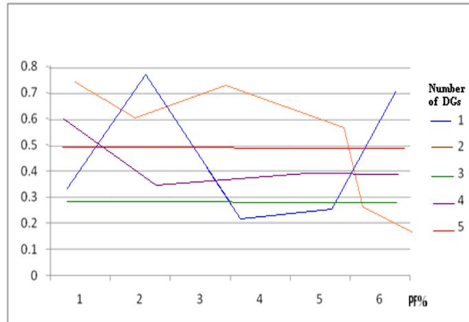
**Fig. 8:** Variation in voltage deviation with optimum number of DGs and Penetrated Factor (PF%).
