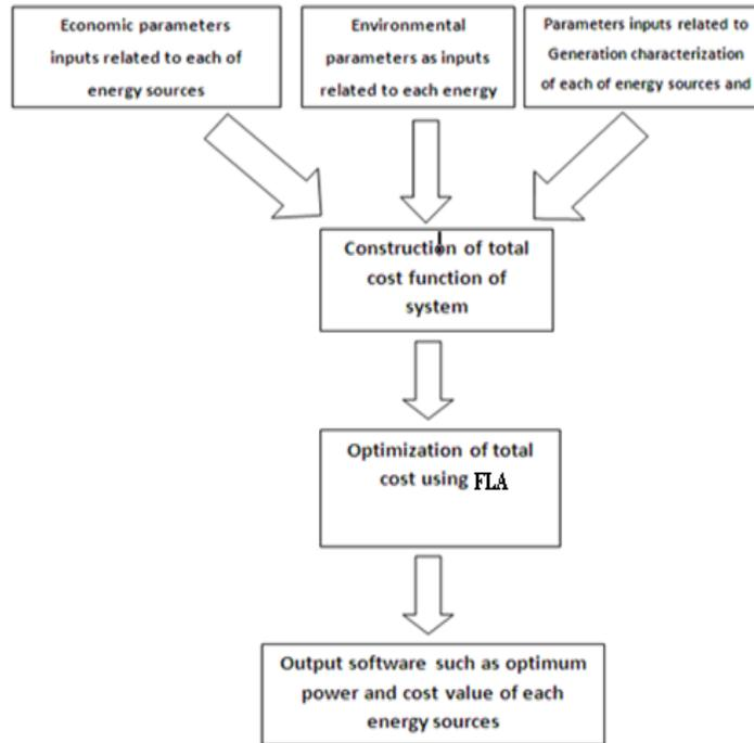
**Fig. 5:** Flowchart of optimization procedure with FLA.
