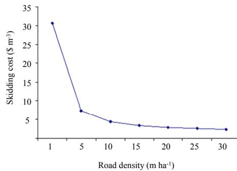
Fig. 4: Skidding cost in different densities of road network for Timberjack 450C.
