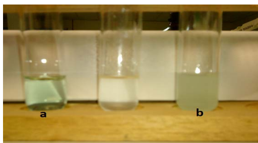
Fig. 9: Biuret test for lipopeptide biosurfactant test. (a) biuret reagent (b) negative result obtained during this study.
