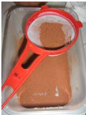
**Fig. 2:** DPK powder sieved to obtain the fine seed powder
