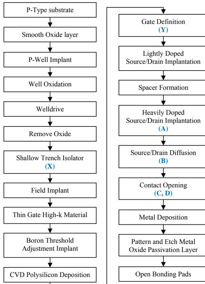
Fig. 3: Complete fabrication process flow. The selection of control and noise factors can then be referred to this figure.
