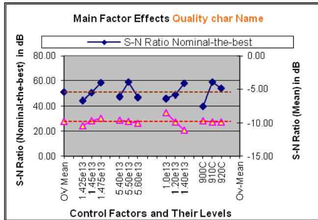
Fig. 3: S/N graph for threshold voltage in NMOS Device
