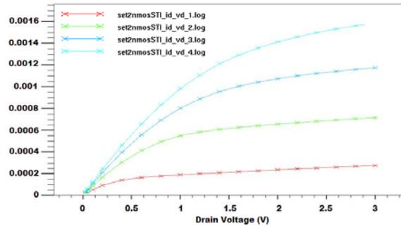
**Fig. 4:**  $I_D$  versus  $V_D$  Relationships
