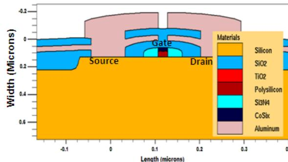
**Fig. 1:** Completed NMOS transistor
