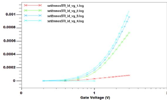
**Fig. 5:**  $I_D$  versus  $V_G$  Relationships
