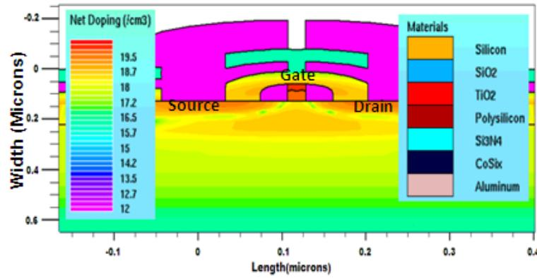
Fig. 2: The doping profile of the NMOS transistor
