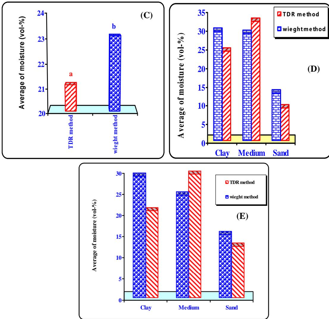
**Fig. 3:** Comparing the moisture using weight and TDR procedures in different soil types:
