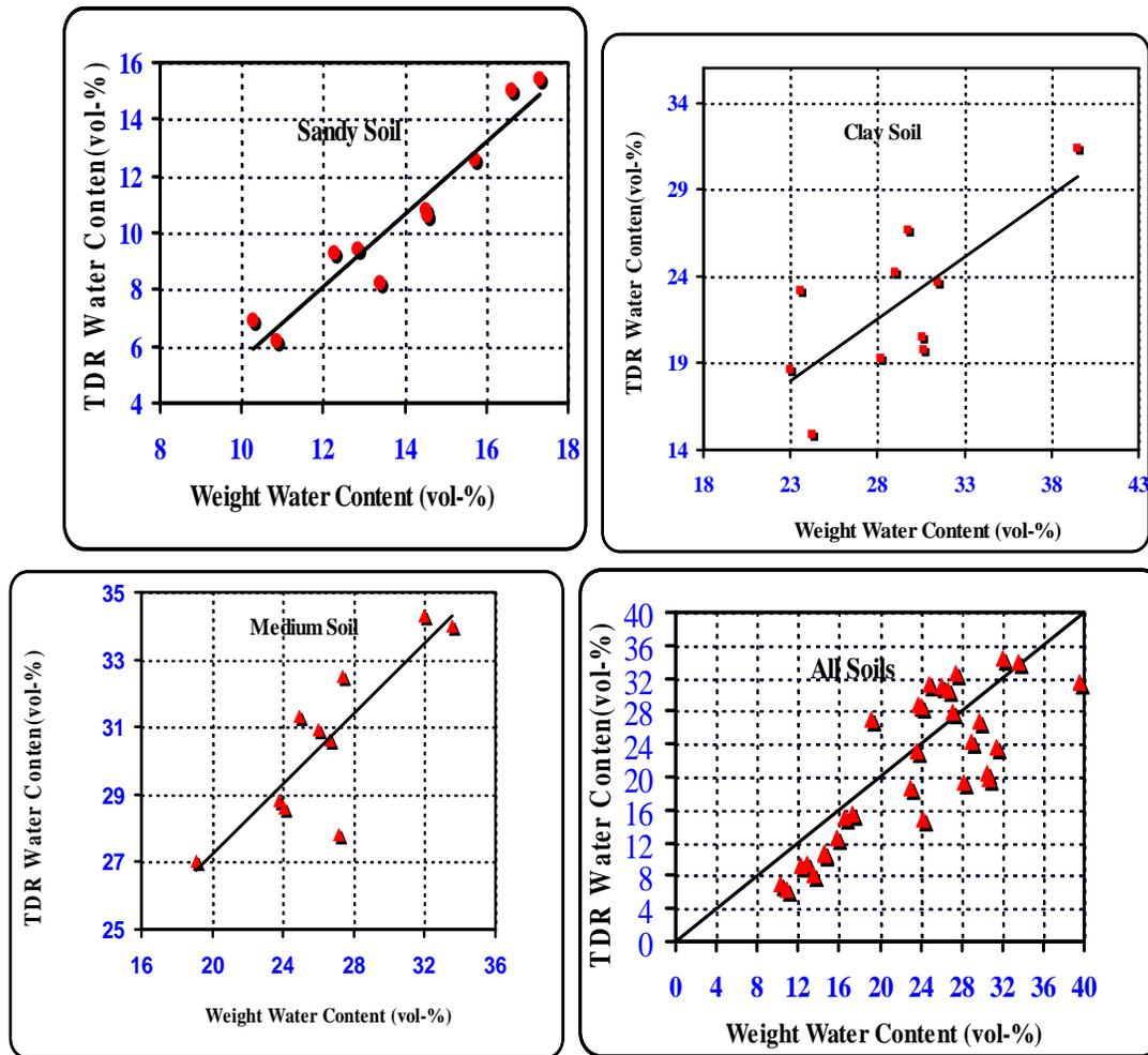
**Fig. 4:** The relation between the average percentages of mass moisture in both weight and TDR procedures
