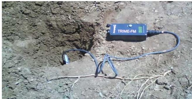
**Fig. 2:** The measurement of soil moisture using TDR set
