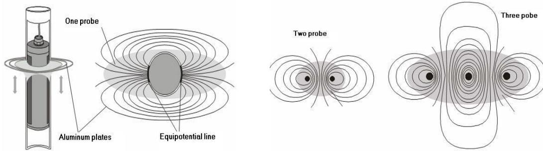
**Fig. 1:** The electrical field around the probes in the states of one, two and three probes
