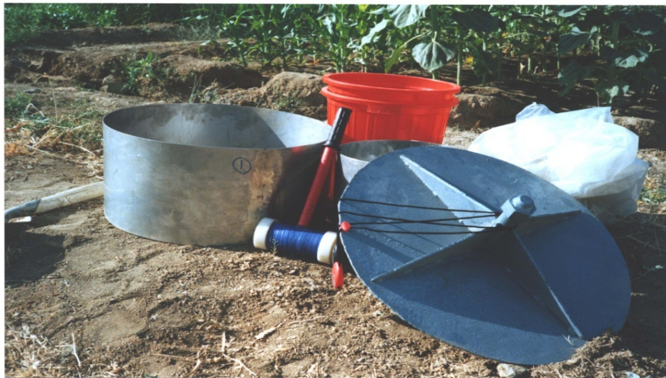
Fig. 1: The needed materials to execute infiltration test in double rings method.
