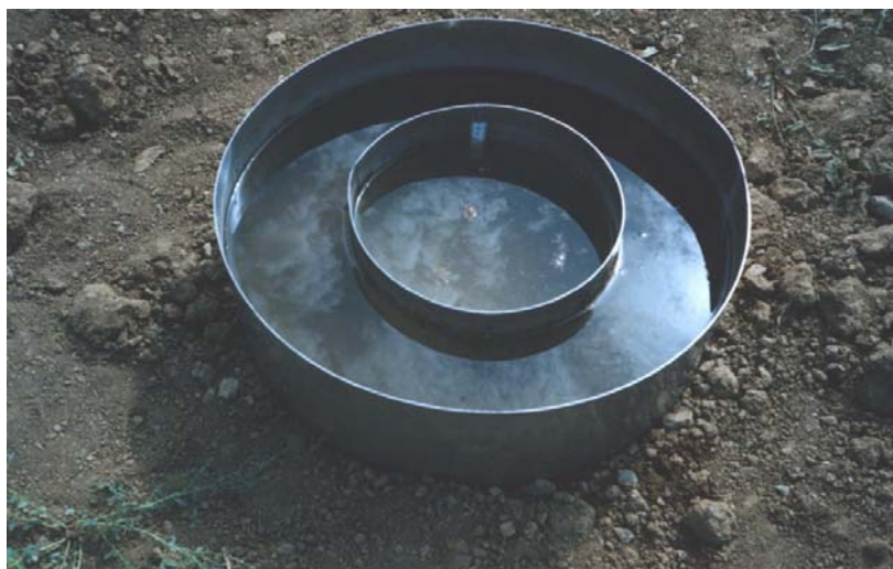
Fig. 2: Ring installing and soil infiltration measuring in the field.
