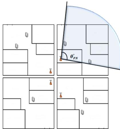
**Fig. 3:** Beamwidth Shaping in Femtocells using Directional Antennas.
