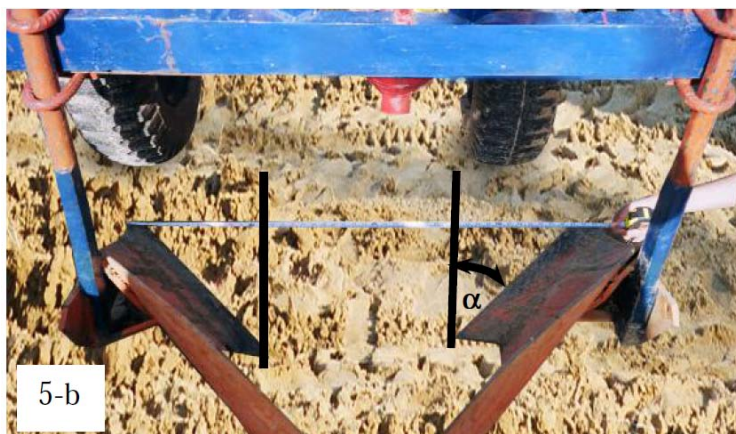
Fig. 5: The setting angle ( \alpha ) of wide raised beds former.
