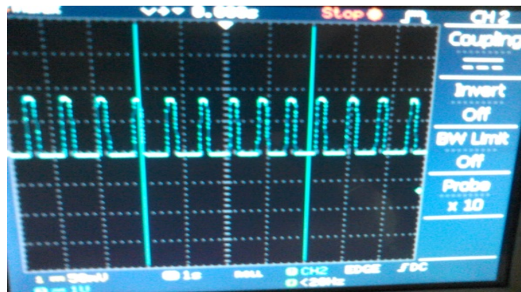
Fig. 3: Output form the Heart-Rate Measuring Circuit
