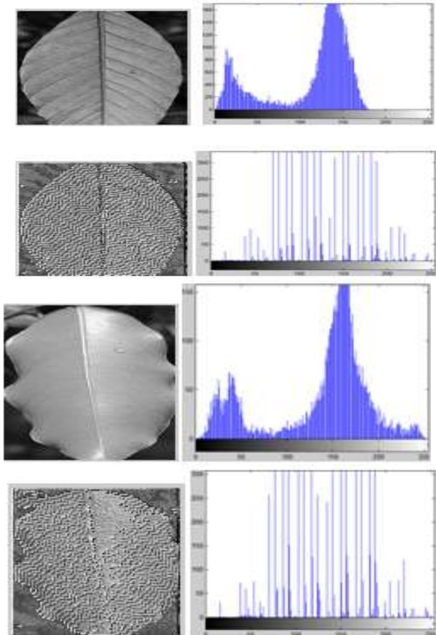
**Fig. 8:** Examples of original images with their corresponding Histograms and new generated images from original images using LGS along with their corresponding Histograms.
