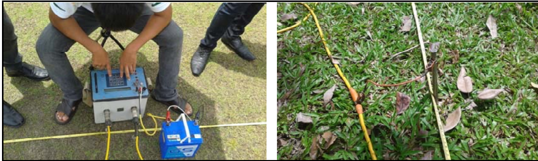
Fig. 6: 2D-resistivity data acquisition.
