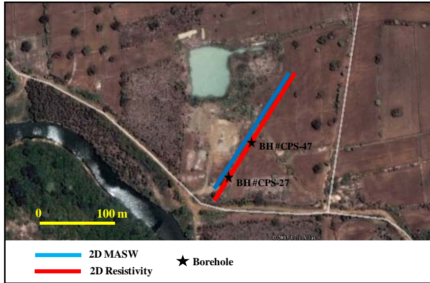
Fig. 2: Location of the geophysical survey line. The 2D-resistivity transect (235 m, shown in red) and 2D-MASW transect (200 m, shown in blue) are actually on the same location (bar the 35 m extra for the 2D-resistivity transect), that shown in red, but the 2D-MASW transect is drawn slightly displaced for clarity of presentation only.
