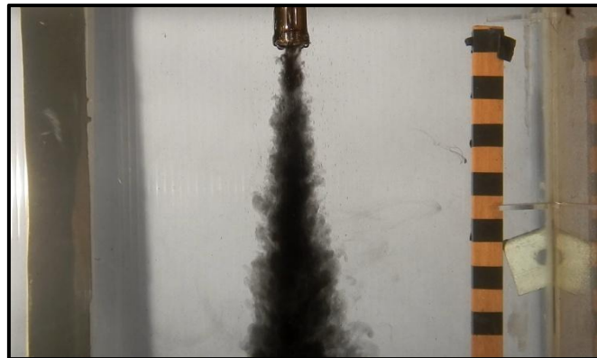
Fig. 2: An RGB image of the flow at 100% valve opening extracted from a video recording.
