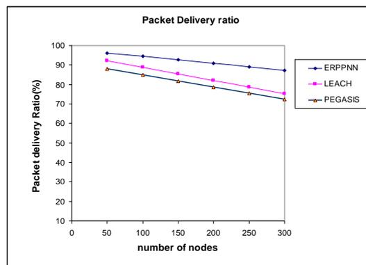
Fig. 3: Packet Delivery Ratio.
