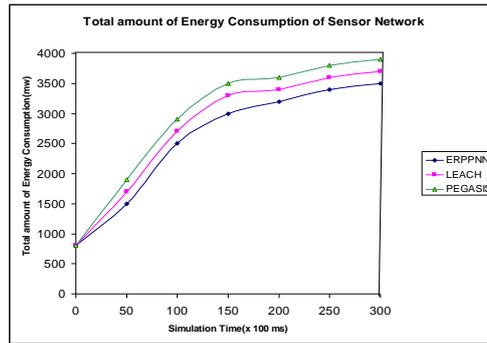
Fig. 2: Total amount of Energy Consumption of sensor networks.
