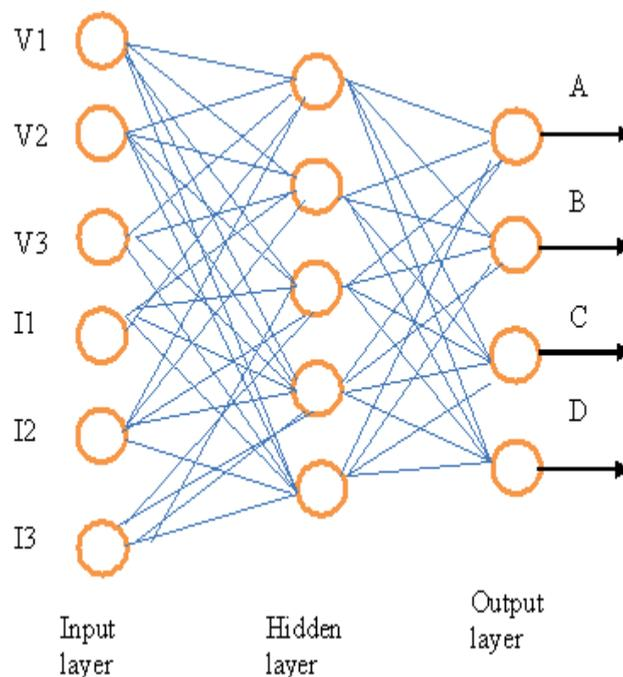
**Fig. 3:** Back Propagation Nn For Fault Classification
