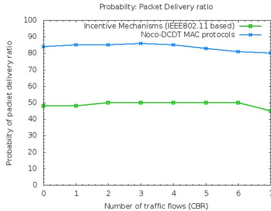
Fig. 10.5: Packet traffic delivery ratio of *Noco-DCDT MAC* Protocols cooperative transmission.
