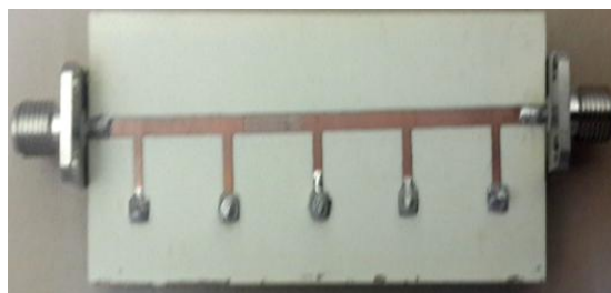
Fig. 8: Photograph of the fabricated UWB BPF integrated with U-shape DMS.
