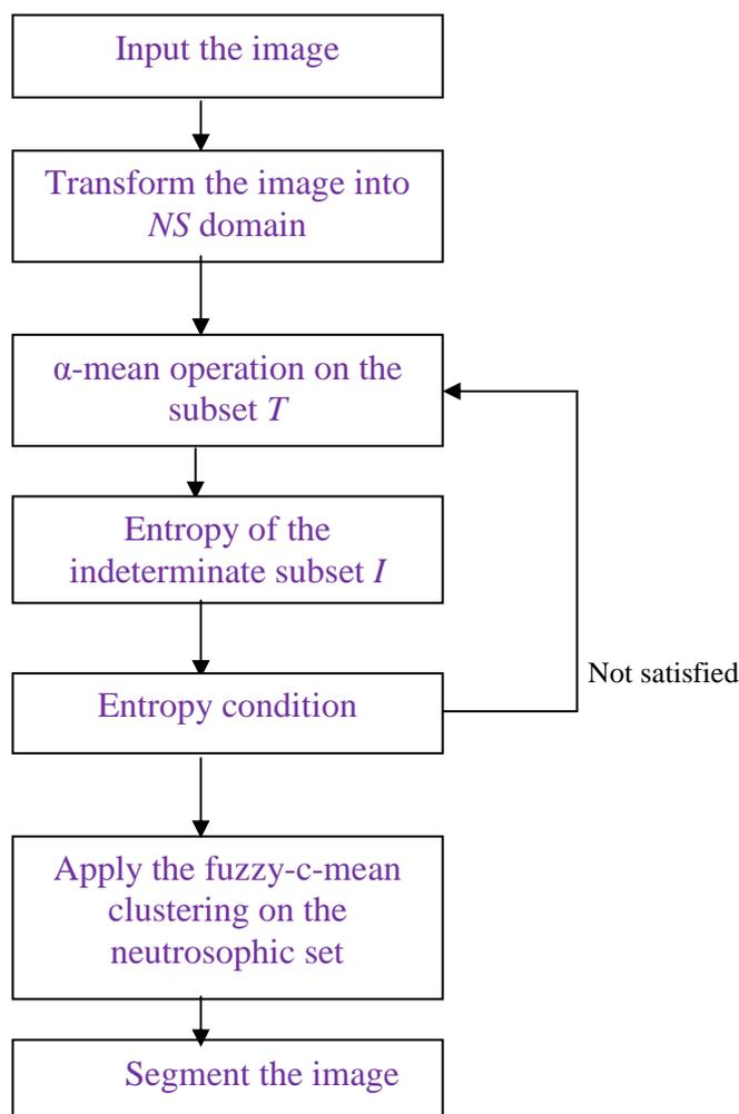
**Fig. 1:** Flow chart of EFCM segmentation algorithm
