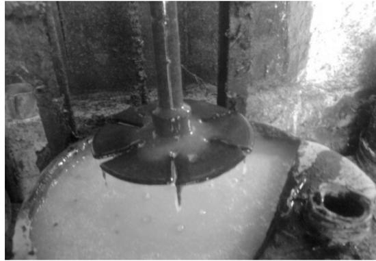
**Fig. 1:** fabricated -Disc impeller
