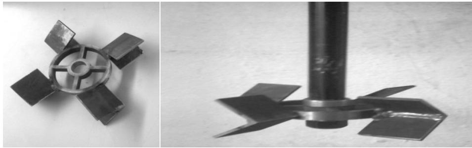
Fig. 6: fabricated parts and assembly of Different impeller blade angles
