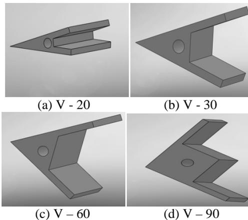
Fig. 5: Different impeller blade angles [a,b,c,d]- Modeling
