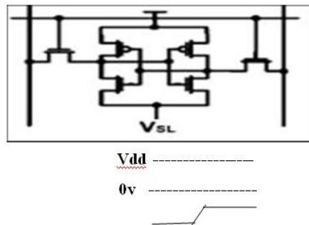
**Fig. 8:** Source biasing technique
