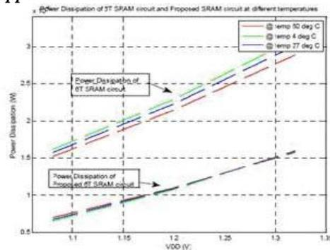
Fig. 19: Power dissipation of SRAM at different temperatures.
