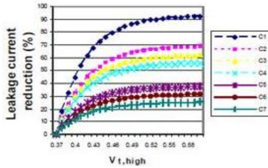
Fig. (15,16): Measured cell leakage during idle and drowsy back bias state Figure 15. Leakage current reduction for each configuration using dual Vt transistors.
