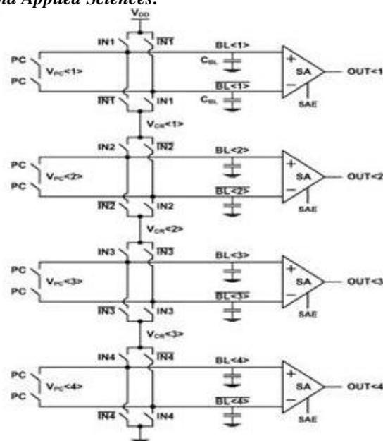
**Fig. 5:** Concept of bit-line charge recycling (n=4).
