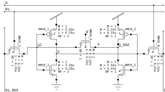
Fig. 3: 7T SRAM cell.
