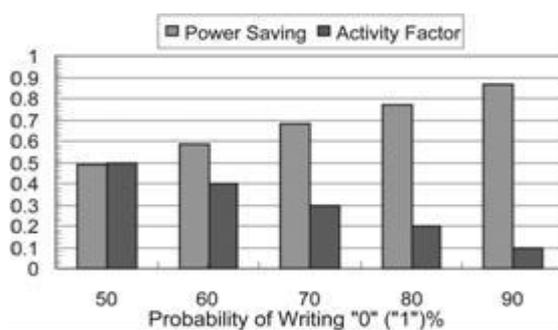
**Fig. 12:** Power saving and activity factor at different writing “0” probabilities using the.
