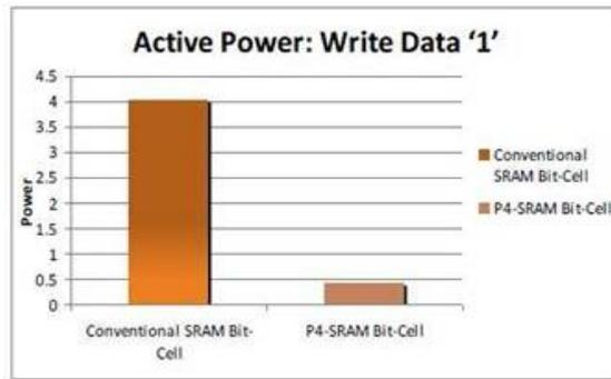
Fig. 17: Active powers for write data“1” using P4SRAM cell.
