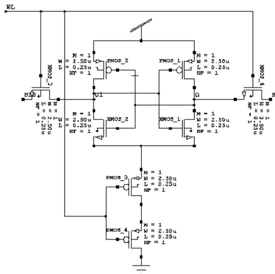
**Fig.7:** P4 –SRAM Bit cell structure.
