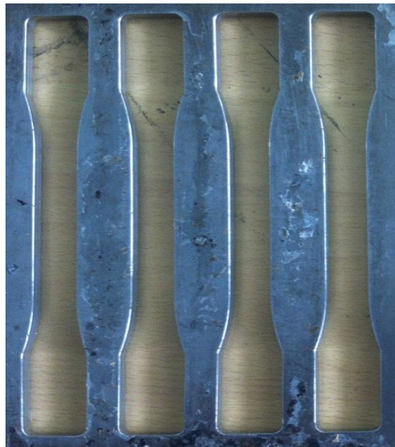
Fig. 2: Tensile test frame made from stainless steel SAE 304.
