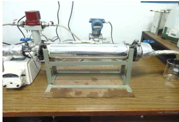
Fig. 2: Experimental Flooding System Set Up.
