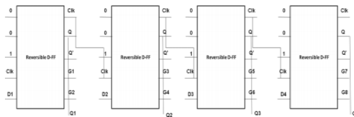
Fig. 16: Parallel In Parallel Out Shift Register using reversible D flip-flop.
