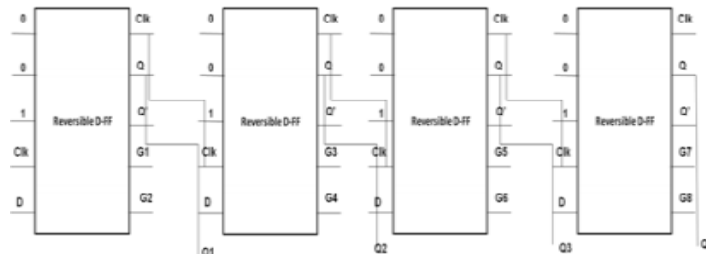
Fig. 15: Serial In Parallel Out Shift Register using reversible D flip-flop.
