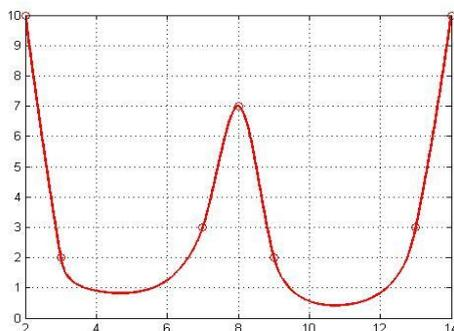
**Fig. 1(c):** Is drawn through using the scheme developed in section III with the values of free shape parameters set as:  $u_i = [0.5, 1, 0.5, 2, 0.5, 1]$   $v_i = [0.5, 5, 0.5, 0.01, 5, 1]$
