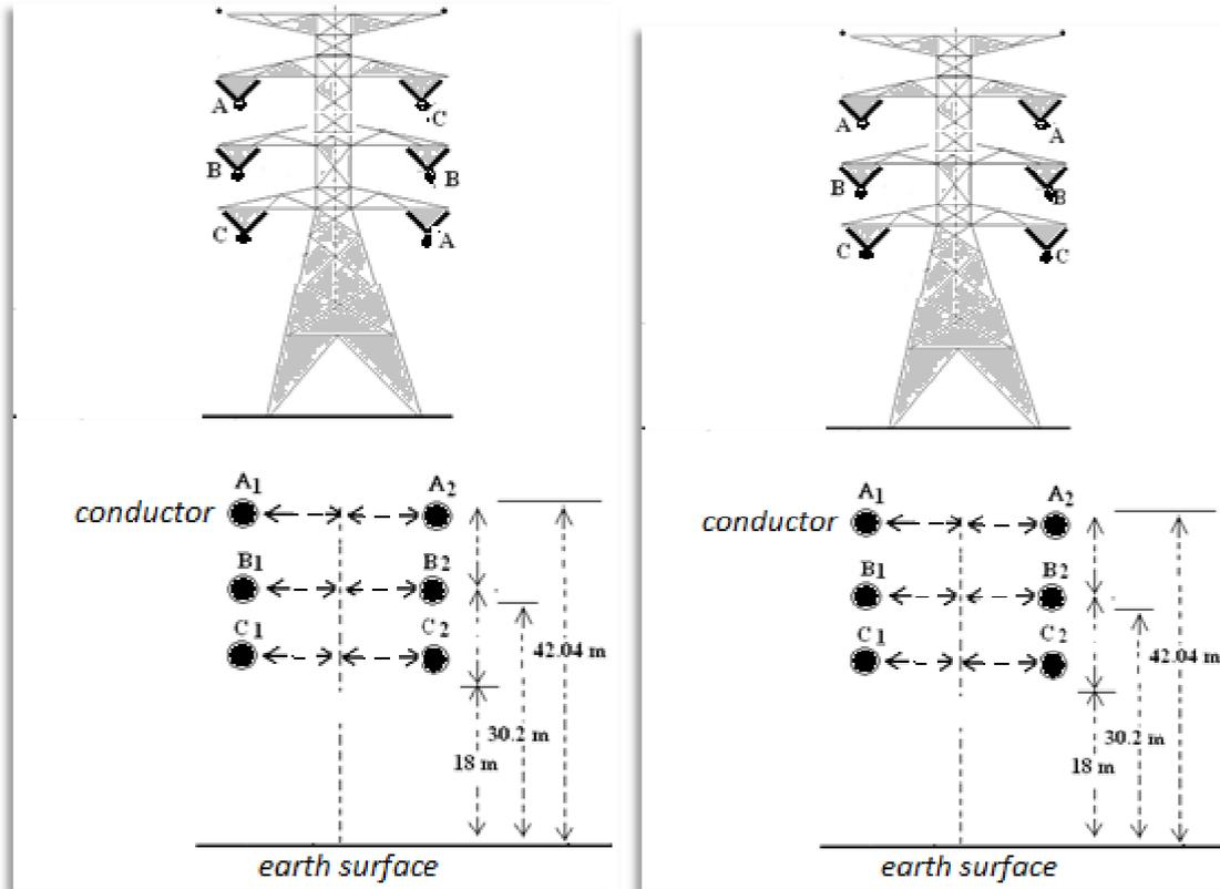
**Fig.2:** Transmission line (132KV)with double vertical configuration.
