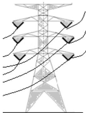
**Fig. 1:** Double circuit vertical configuration transmission line (132 KV).
