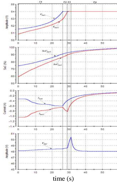
**Fig. 7:** Simulation result when Microgrid changes from Mode I to Mode II.
