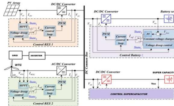
**Fig. 3:** DC Microgrid with control loops.
