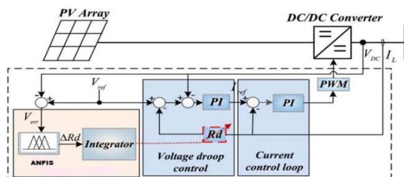
**Fig. 6:** Proposed ANFIS controller based virtual resistance for RES under Mode II operation.
