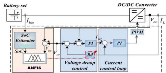
**Fig. 5:** Proposed ANFIS controller based virtual resistance for ESS under Mode I operation.
