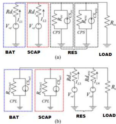
**Fig. 4:** Proposed microgrid operation (a) Mode I (b) Mode II.
