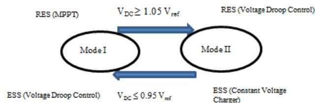
Fig. 2: (i) Mode I - regulated by Distributed ESS.
