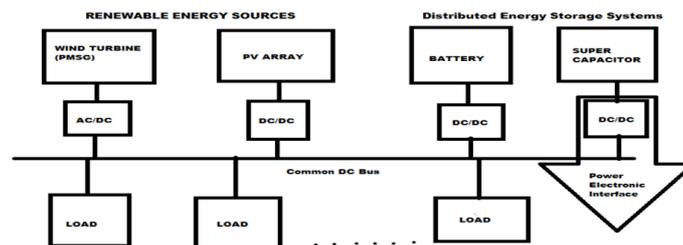
Fig. 1: General Structure of a DC Microgrid.
