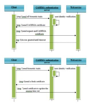
Using the CASHMA application, the client contacts the CASHMA authentication server. The first step consists in acquiring and sending at time *t*0 the data for the different biometric traits, specifically selected to perform a strong authentication procedure (step 1). The application explicitly indicates to the user the biometric traits to be provided and possible retries.
