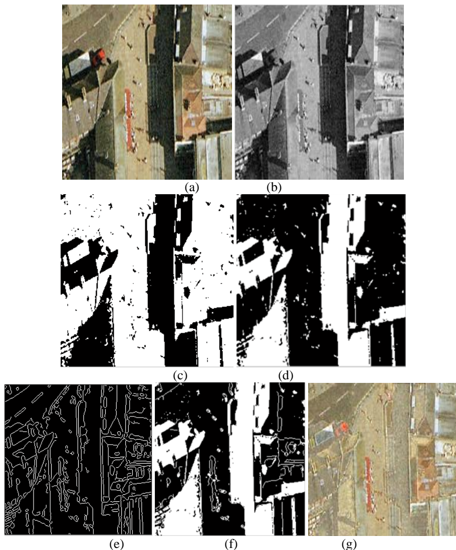
Fig. 5: Final Restoration results for the first MS satellite image. (a) Original MS image of a sub-urban area. (b) Grayscale version. (c) Binary Mask. (d) Complement image for the binary mask. (e) Canny Edge detected image. (f) Super-imposition of edge detected image and complemented image. (g) Recovered image of the proposed system.
