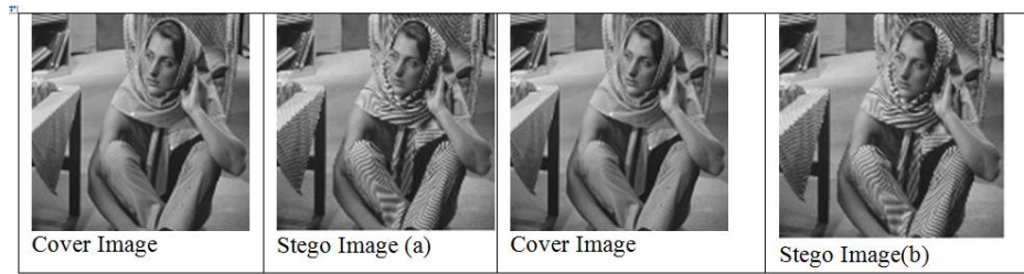
Fig. 2: Cover image is Barbara.bmp (512x512) a)stego image with 256x256 cameraman embedded b)stego image with 256x256 lena embedded.
